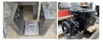
These pictures show the reconditioned Wakefield lubricator and a close up view of one of the four machined axle box housings.
